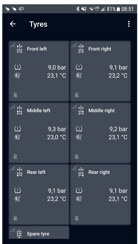
Figure 14: Detail view of the tyre status with pressures and temperatures for each tyre
