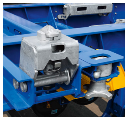
With 2x20' loads the two KLAPP LOCKS serve to lock the rear end of the front container.
