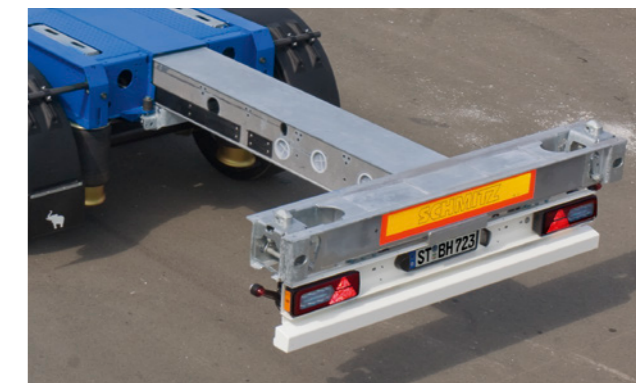
The rear extension pneumatically extends to the selected container position.
