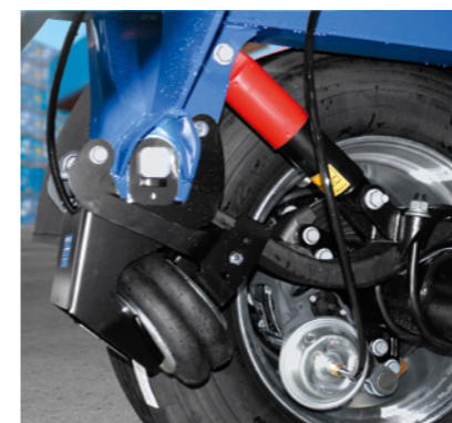
The lift axle * as a starting aid extends the wheelbase and, thus, increases the pressure on the drive axle.
