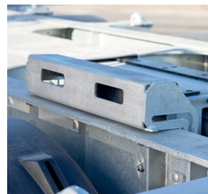
Three pairs of folding container supports* for containers without tunnel.
