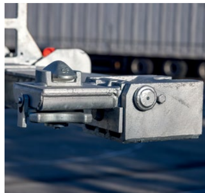
Folding lock on the rigid front bar in the twist lock position.
