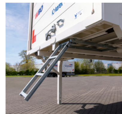
Galvanised steel folding ladder for access to the load compartment.
