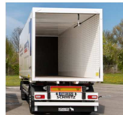
Open roller shutter* in interchangeable case for fast loading cycles, quick access at the ramp and in confined spaces.
