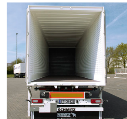
Opened double wing door with an opening angle of 270°. Close-fitting to the side wall for good manoeuvrability.
