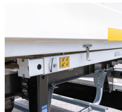
Support leg 90° in transport position with safety catch.
