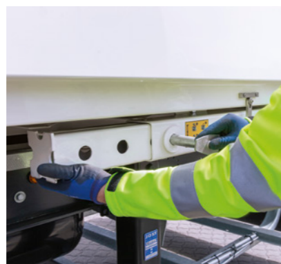
Adjusting the telescopic support leg* for the semi-mounting heights of 1,120 mm, 1,220 mm and 1,320 mm.
