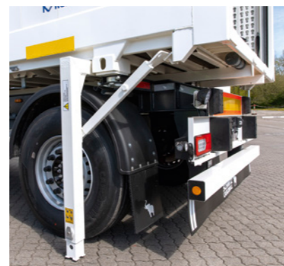
Four support legs with diagonal securing according to DIN EN 284 (as standard version with fixed fifth wheel height of 1,320 mm). Four receptacles for securing with twist locks according to coding profile C30.
