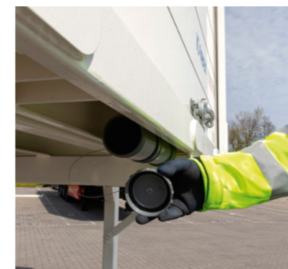
Document tube* for accompanying documents mounted on the underside of the rear.
