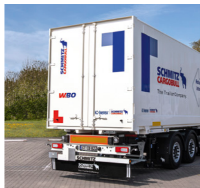
Double folding door with robust, external espagnolette locks. When open, the doors are secured with a chain.
